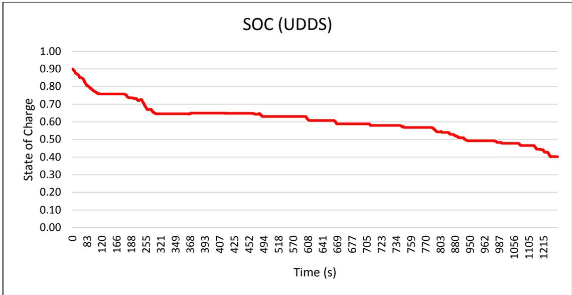
FIGURE 5.4: SOC in battery pack (UDDS)
