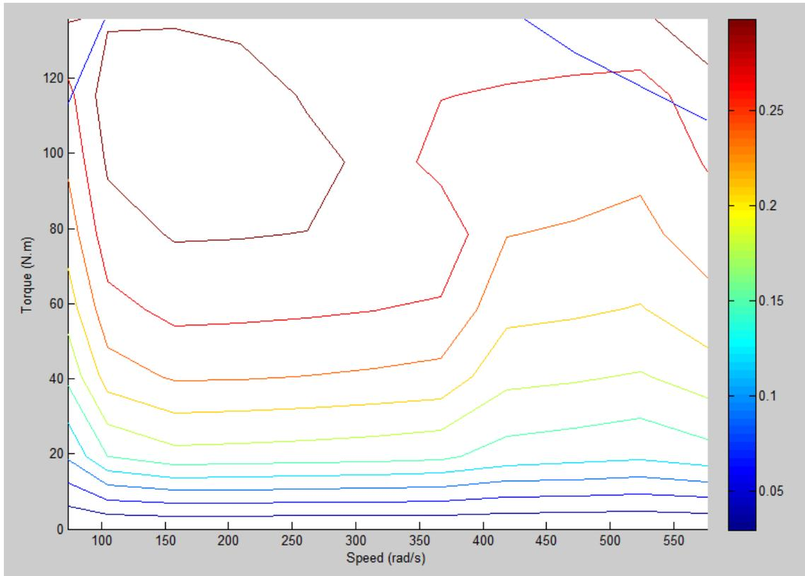
FIGURE 4.19: ICE efficiency
