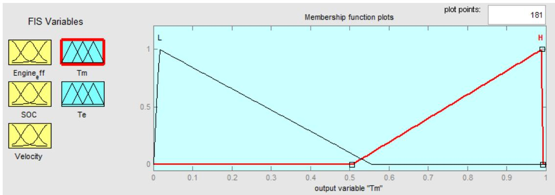
FIGURE 4.24: Torque motor output
