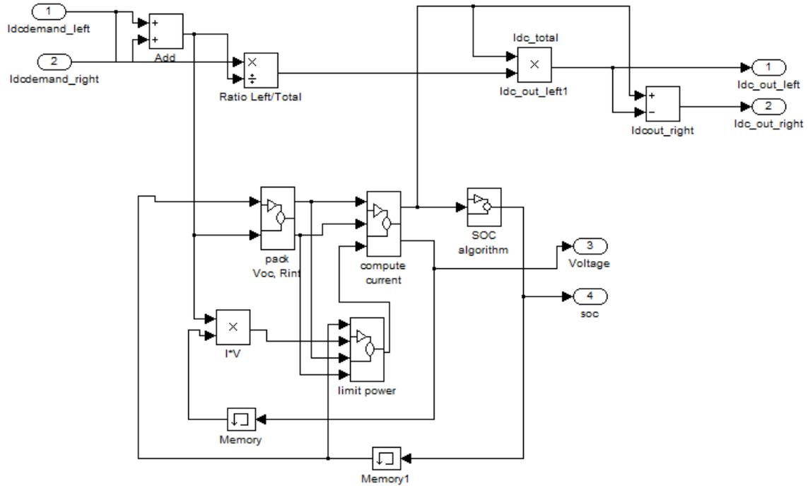
FIGURE 4.26: Battery pack model
