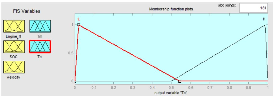
FIGURE 4.25: Torque engine output
