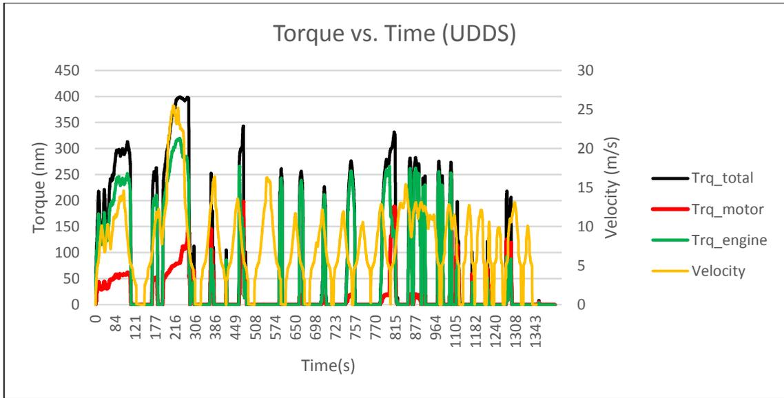
FIGURE 5.1: Torque distribution in HEV model (UDDS)
