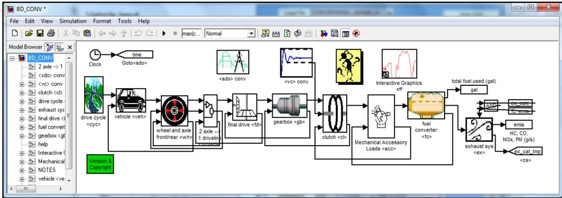
FIGURE 4.11: Vehicle model Block Diagram developed in ADVISOR
