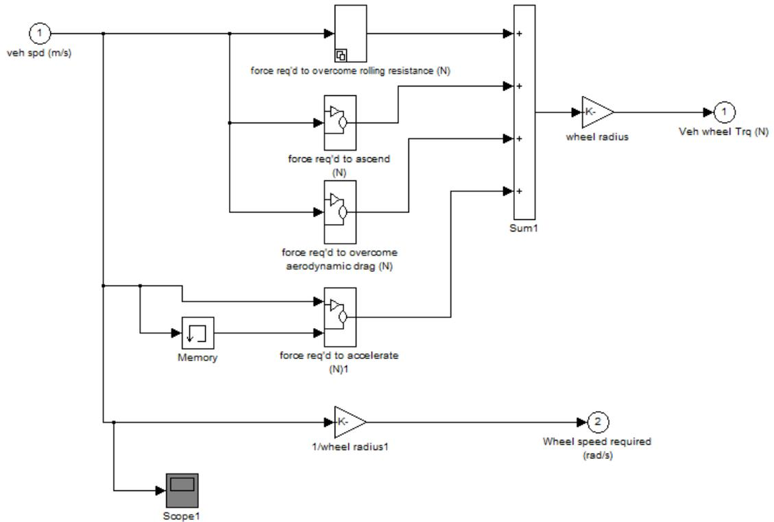
FIGURE 4.4: Vehicle requirement block model
