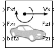
FIGURE 4.7: Longitudinal Vehicle Dynamic block
