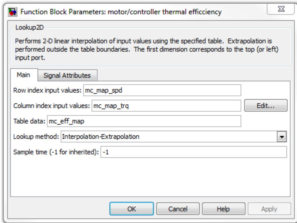
FIGURE 4.28: Look-up table for motor thermal efficiency
