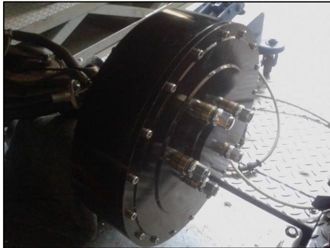
FIGURE 2.1: In-Wheel Motor
