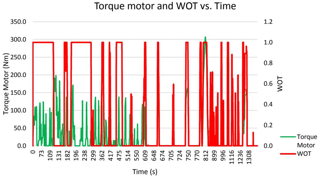
FIGURE 5.3: Torque distribution to motor according to WOT
