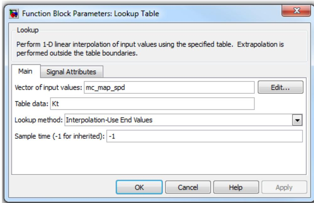
FIGURE 4.27: Motor torque constant look-up table
