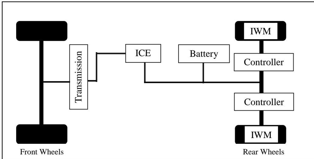
FIGURE 1.3: Parallel configuration of components in HEVs [10]
