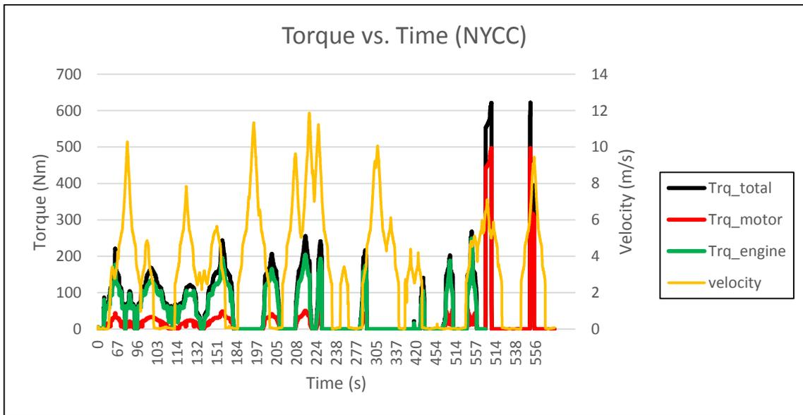
FIGURE 5.2: Torque distribution for HEV model (NYCC)
