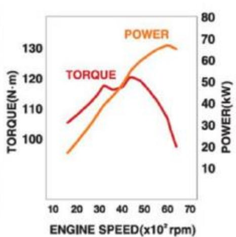
FIGURE 4.5: Graph of Torque and Power VS Engine Speed. [13]
