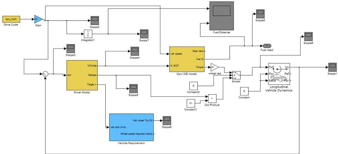
FIGURE 4.1: Overview of conventional base vehicle model
