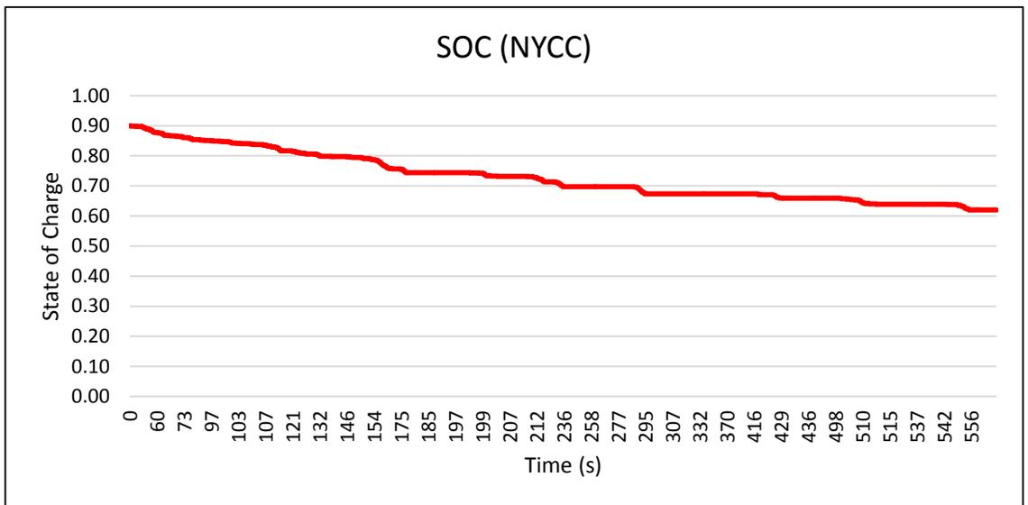
FIGURE 5.5: SOC in battery pack (NYCC)
