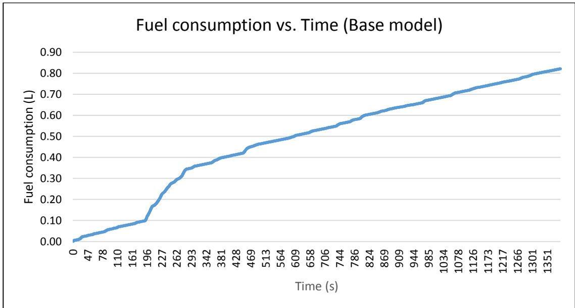
FIGURE 5.7: Fuel consumption for base vehicle model (UDDS)
