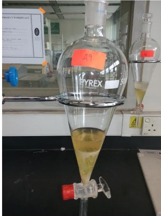
Figure 9 The transesterified oil is settled for overnight
