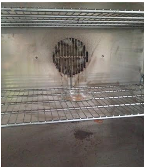
Figure 5 The Catalyst is dried in the oven for 110°C for 12 hour
