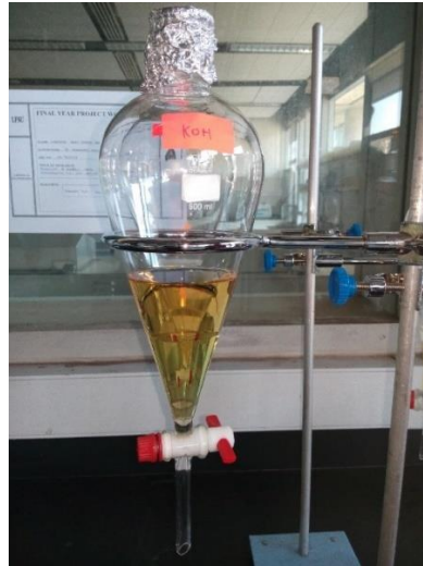
Separation of Biodiesel and Glycerine in Separating Funnel
