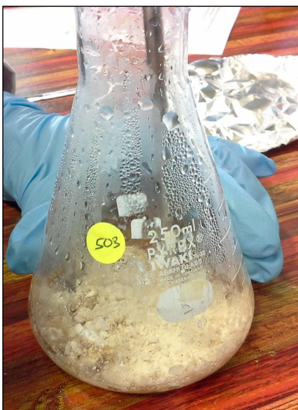
Figure 9: Sample 503, a sample with higher ionic liquid content which became hard and stick to the glass container
