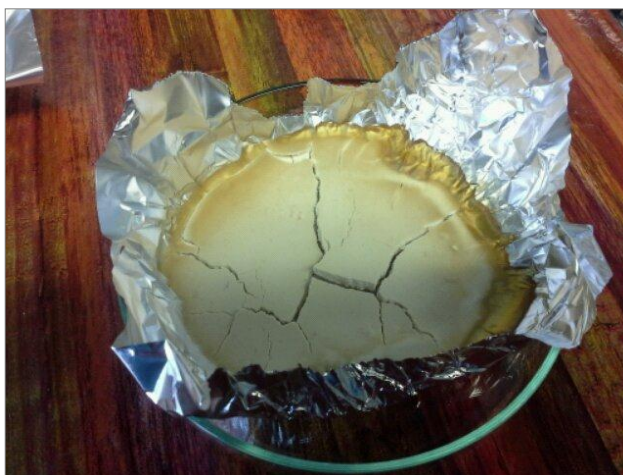
Figure 10: Non-homogenized Mixture of Starch & Plasticizer After 24hours of Drying at 55°C
