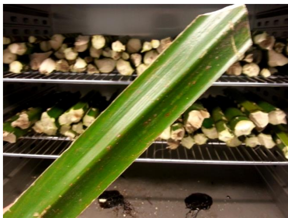
Figure 8: The photo of washed OPF which has been cut and ready to be dried at drying oven
