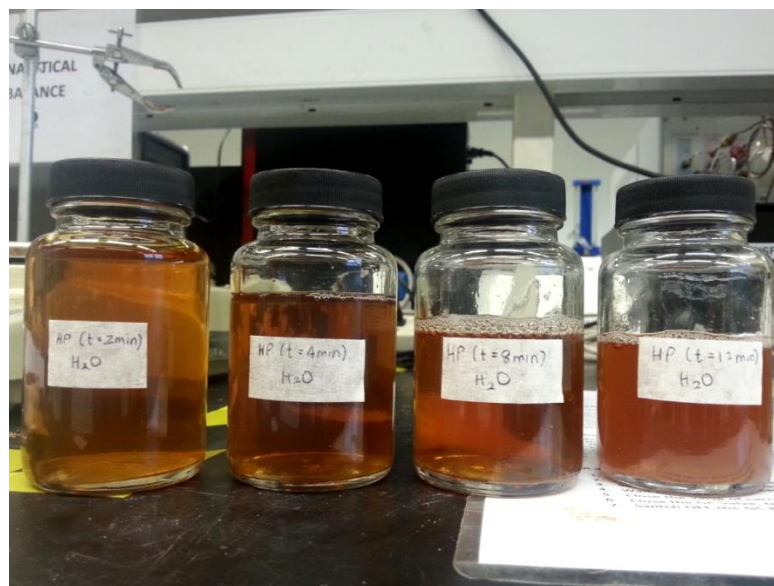
Figure 11: The photo of pre-treated sample (filtrate) at 0 N of NaOH
