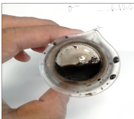
FIGURE 4.9. Biodiesel Produced from Dried Microalgae Biomass through Transesterification Reaction
