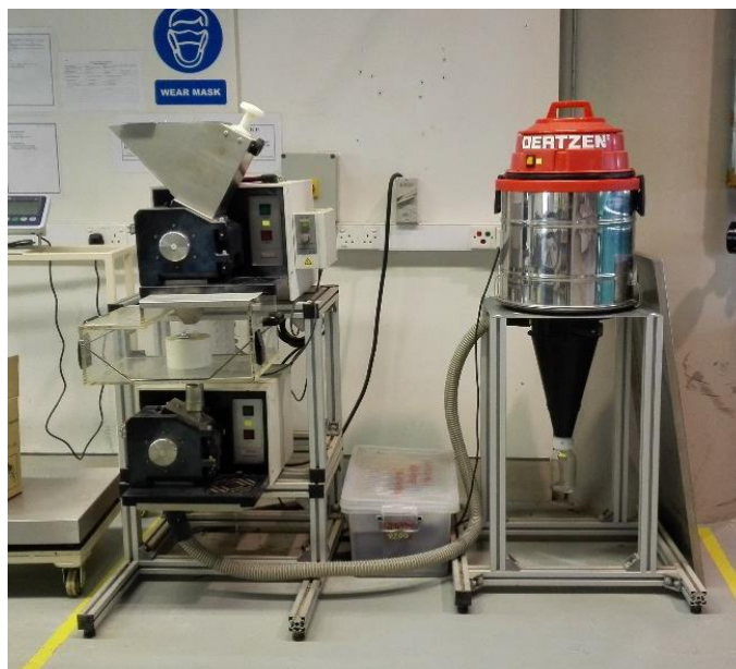
FIGURE 10. Grinder and Siever Used to Crush RSS Sample
