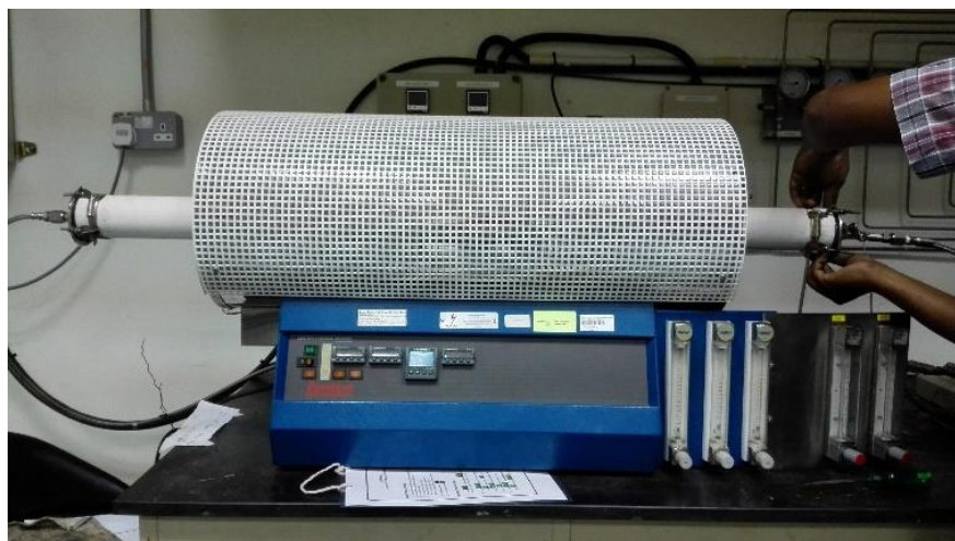
FIGURE 13. Tube Furnace Used for Activation and Carbonization
