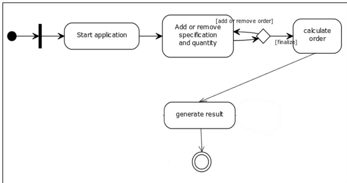
Figure 3.4 Activity diagram for Calculate Order use case
