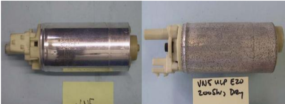
Figure 2: Corrosion on fuel pump surface resulting from immersion into E20 (left)
