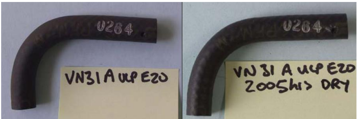
Figure 1: Fuel line before (left) and after immersion testing with E20
