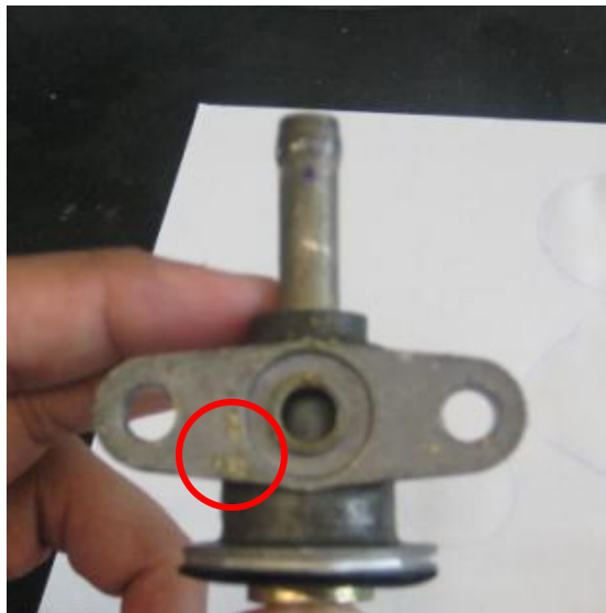
Figure 8: Corrosion at fuel regulator (E85)
