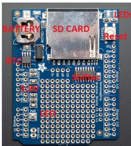
Figure 14- SD Card Shield
