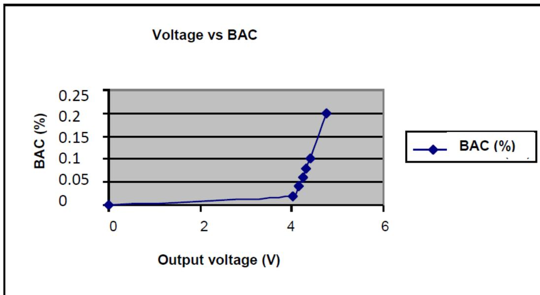
Figure 17 – Response Curve of BAC (%) to Voltage Values
