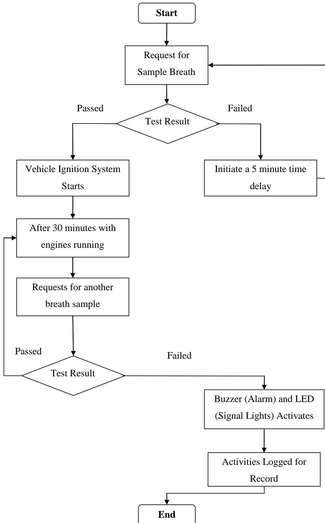
Figure 3 – Flowchart of Process Flow for Breathalyser Ignition Interlock
