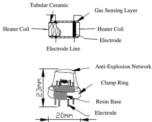
Figure 11 – MQ-3 Alcohol Sensor
