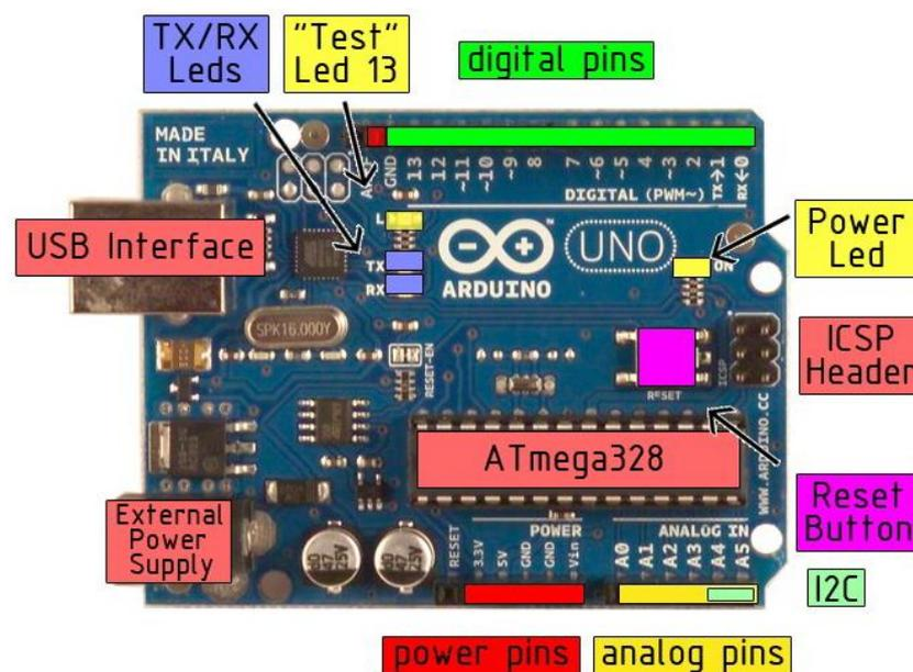
Figure 13 – Arduino Uno Microcontroller Board
