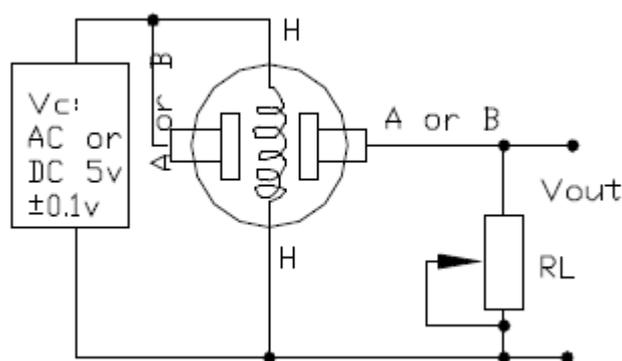
Figure 12 – Circuit Diagram of MQ-3 Alcohol Sensor
