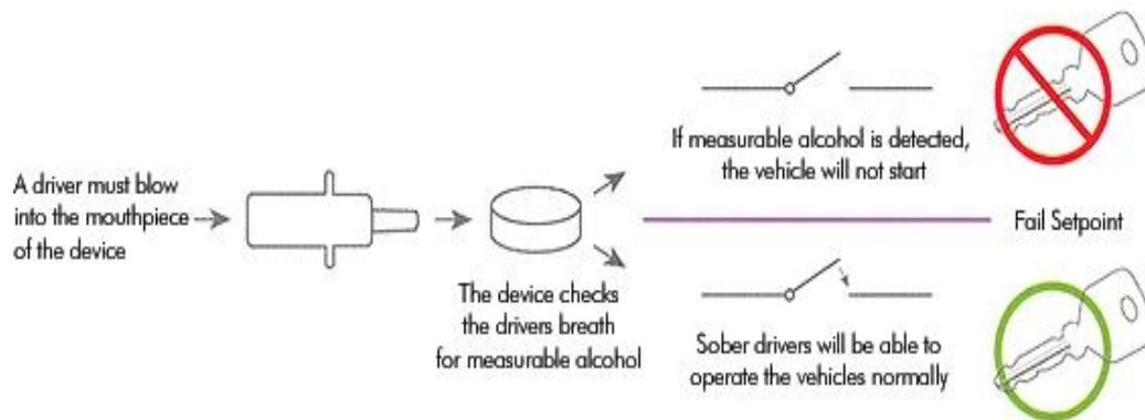
Figure 4 – Block Diagram of Process Flow in Breathalyser Ignition Interlock
