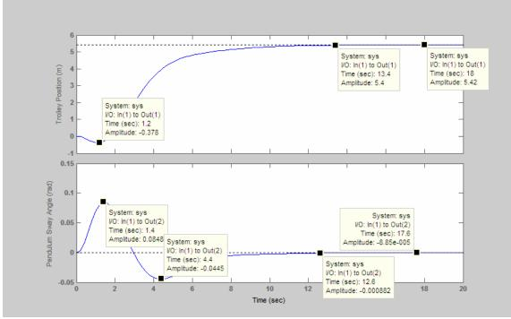
**Figure 22**: Response for Controller with  $m_L$ =50t
