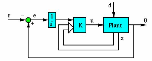
Figure 14: Closed-Loop System with Integral Action
