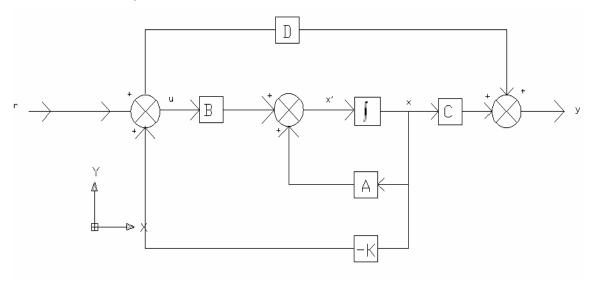
Figure 2 : State Variable Feedback Control System
