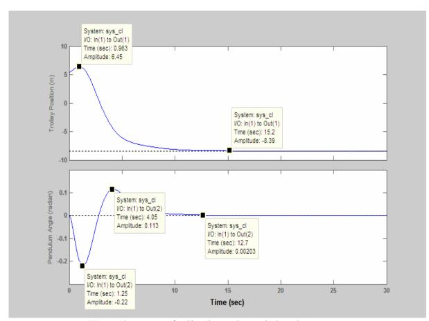
Figure 13: Response for Closed-Loop System in State Space
