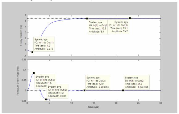
**Figure 20**: Response for Controller with  $m_L$ =0.05t
