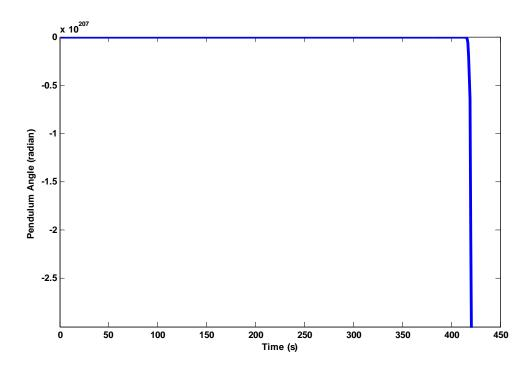
Figure 11: Response for Sway Angle, in Open Loop System in State Space
