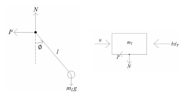
Figure 8: Free-body diagram of the simple pendulum system [26]
