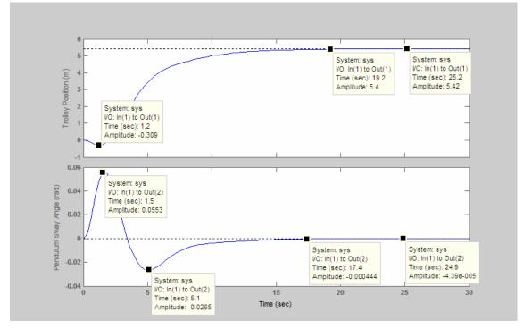
**Figure 19**: Response for Controller with *l*=8m
