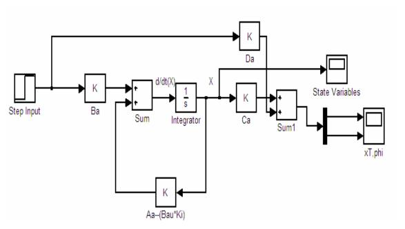
Figure 15: Block Diagram for Closed Loop System with Integral Action
