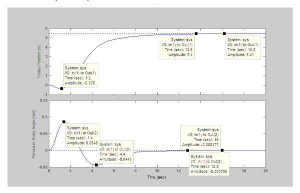
**Figure 21**: Response for Controller with  $m_L$ =5t
