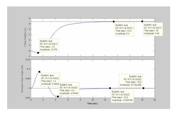
**Figure 23**: Response for Controller with  $m_L$ =500t
