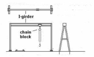
Figure 1 : Basic Structure of Gantry Crane [6]
