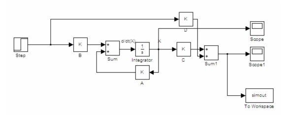
Figure 9: Block Diagram for Open Loop System in State Space
