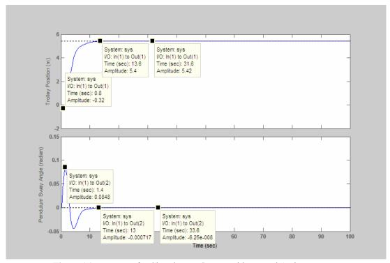
Figure 16: Response for Closed-Loop System with Integral Action
