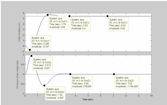
**Figure 17**: Response for Controller with l=1m
