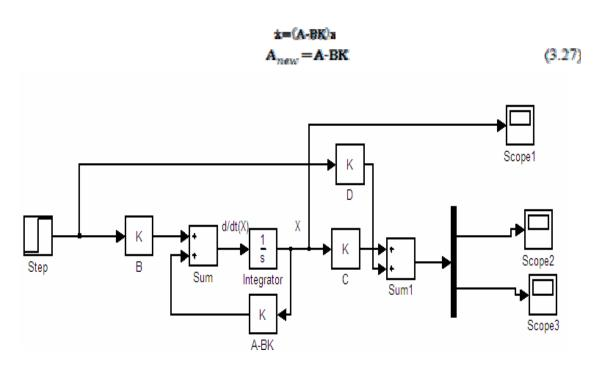
Figure 12: Block Diagram for Closed-Loop System in State Space
