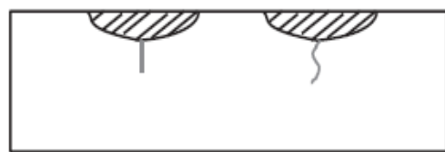
(c) Cracks initiated from localised corrosion
