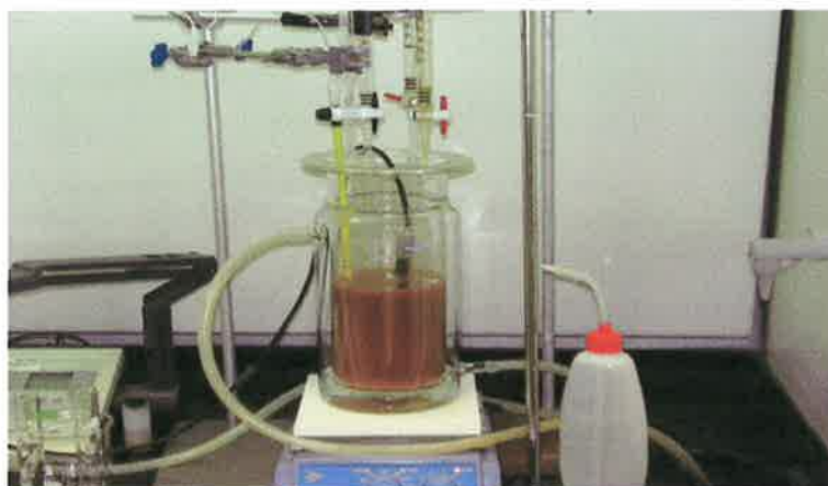
Figure 1 : Degradation of MDEA process by Fenton's Reagent
