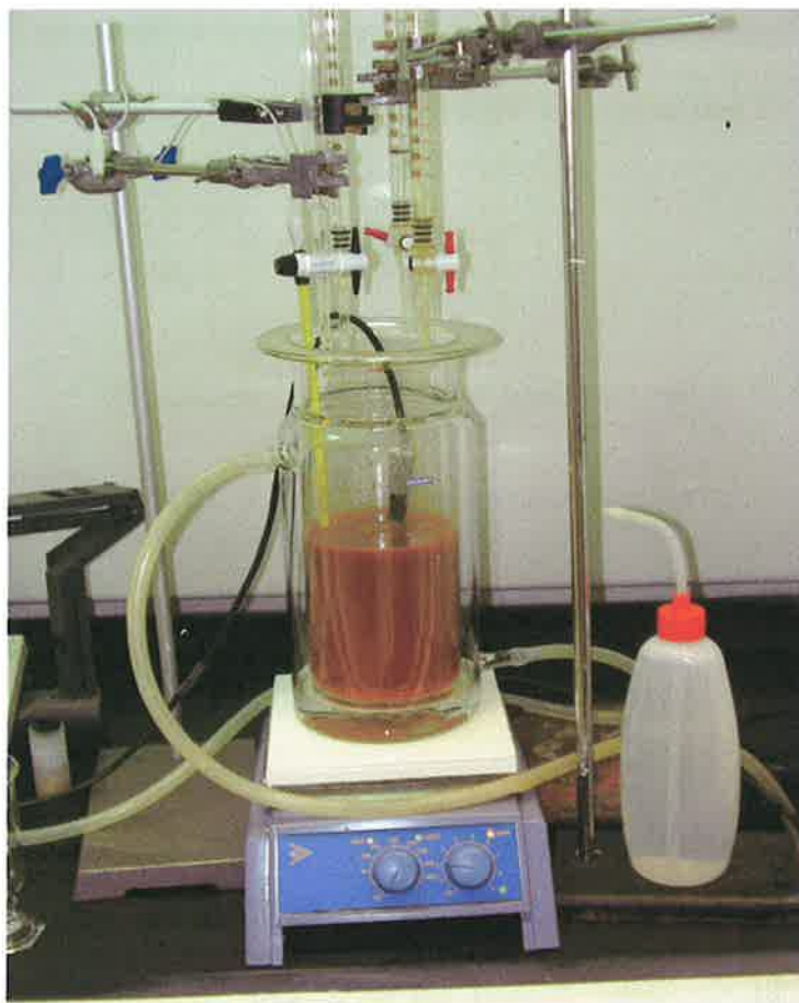
Figure 5 Fenton's Process experimental set up
