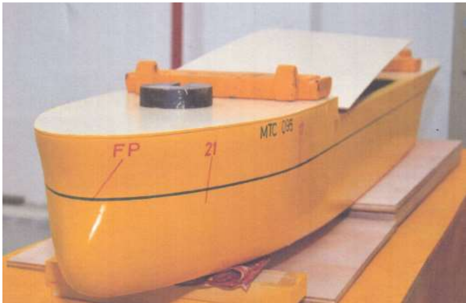
Berantai FPSO model which is ready to be tested.
