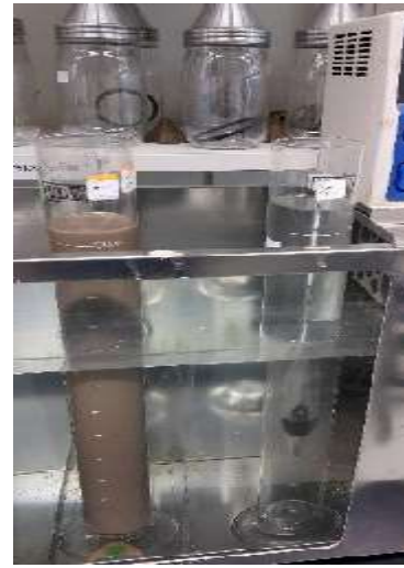
Figure 3.3: one litre of cylinder will be used in hydrometer test
