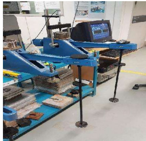
Figure 3.7: Small weight were added during saturation process
