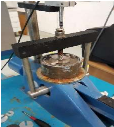
Figure 3.6: Sample were left for saturation stage for 24 hours
