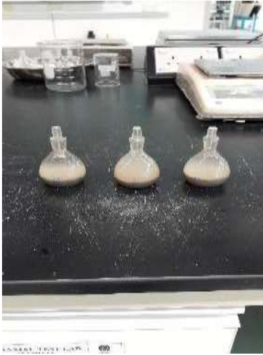
Figure 3.2: Small pyknometer jar will be used in specific gravity test
