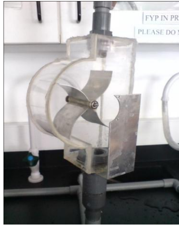
Figure 26 Turbine test without generator
