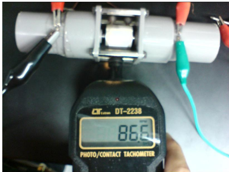
Figure 24 Testing speed for open circuit test
