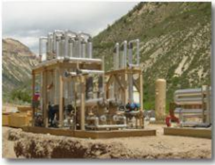
Figure 10: Recovery of CO 2 from associated gas in enhance oil recovery (EOR) programs (Acid gas removal from natural gas)
