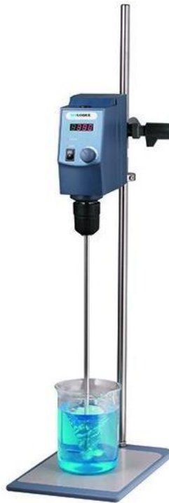
Figure 3: Stirrer in Beaker for Emulsification
