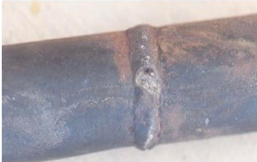
Figure 2.19: Formation of Hole Around Weld Area (A.U. Malik, 2013)
