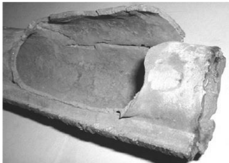
Figure 2.24: Evaporator Tube Window Fracture (M.Djukic, 2005)
