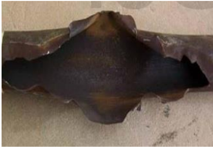
Figure 2.17: A ruptured Economizer Tube due to Fireside Corrosion (A.U. Malik, 2013)
