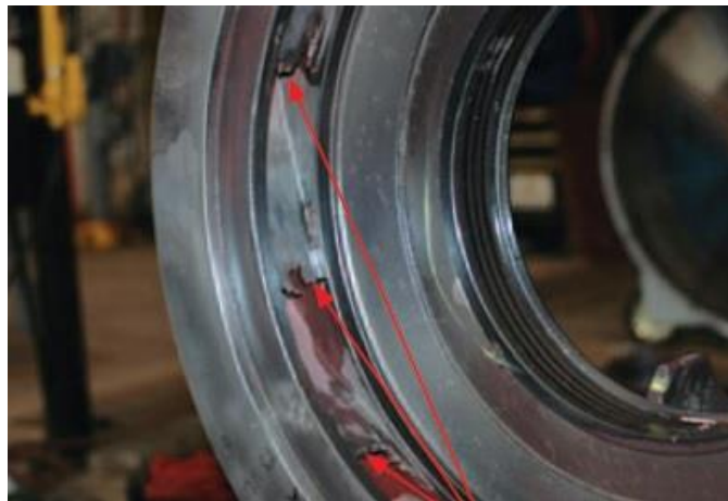
Figure 2.25: Cavitation Signs on Pump's Diffuser (Flowserve, 2010)
