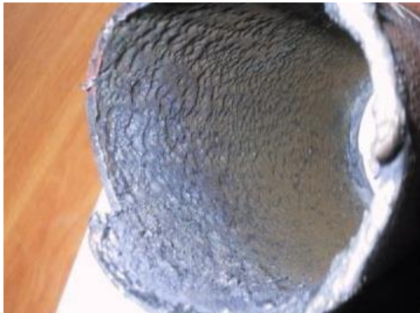
Figure 2.14: FAC attack on tube wall (R.M Sharip,2007)
