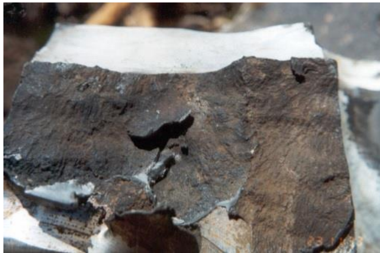
Figure 2.16: Corrosion Fatigue on a Steam Drum, (K.B. McIntyre, 2002)
