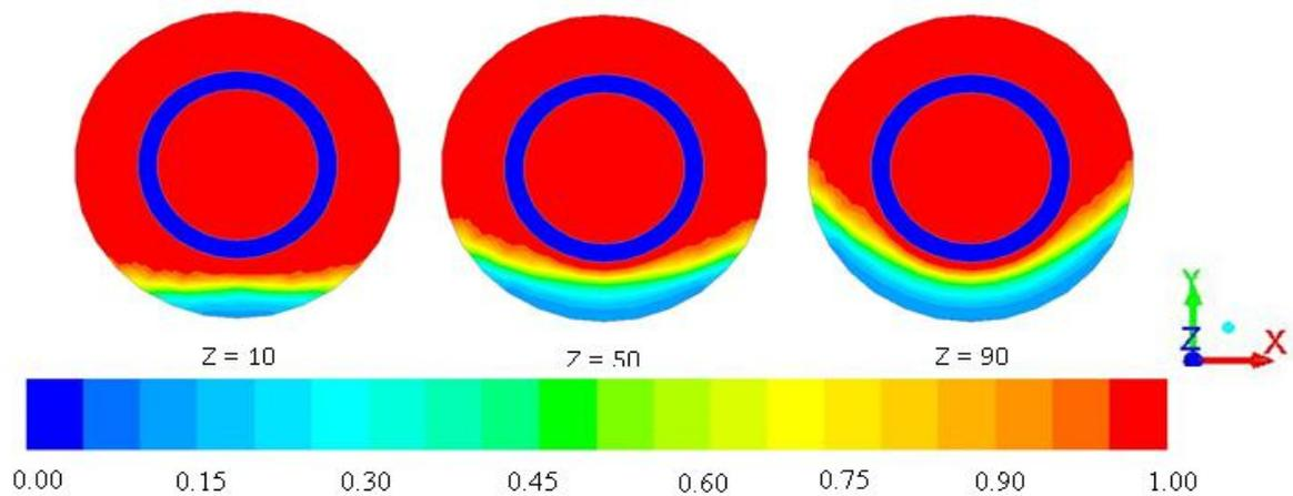
**Figure 10: Effect of horizontal orientation on the liquid fraction**
