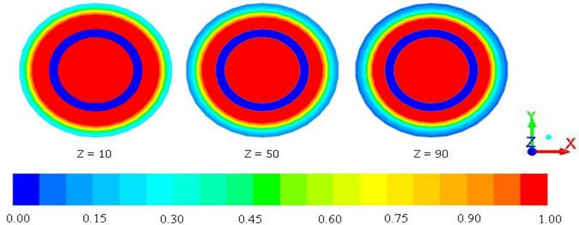
**Figure 8: Effect of vertical orientation on liquid fraction**
