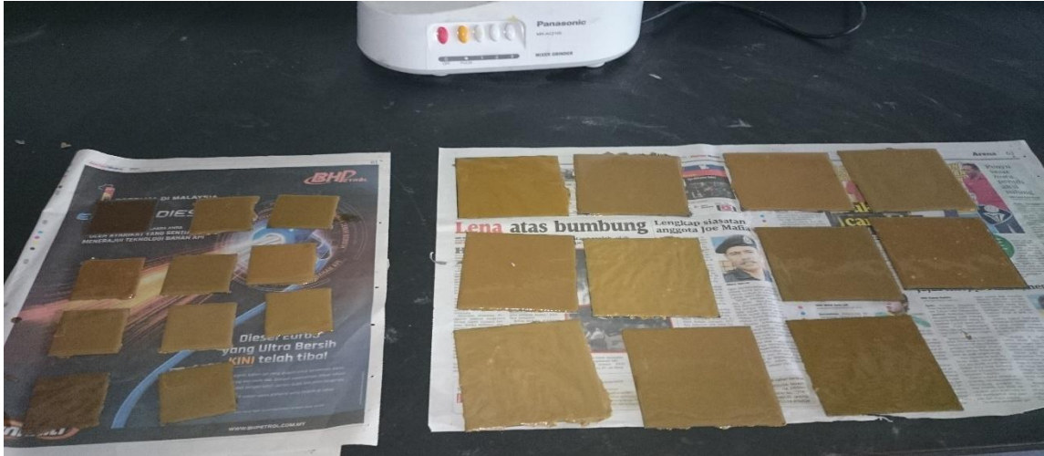
Figure 5: Intumescent coating after fully cured
