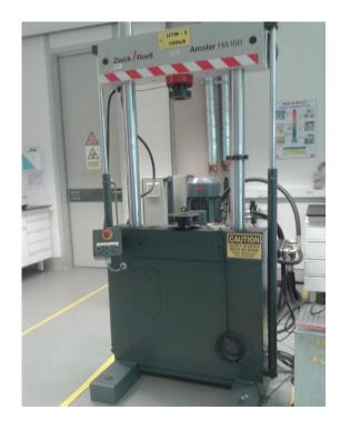
Figure 13: Universal testing machine as static loading device
