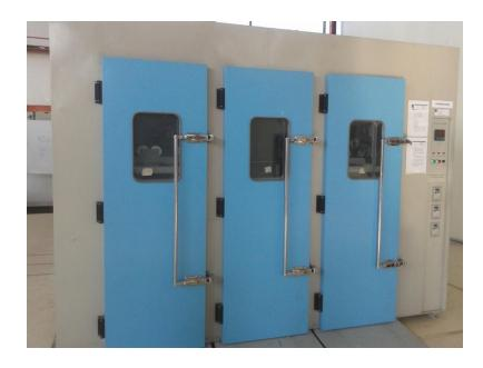
Figure 9: Cure oven for epoxy curing process
