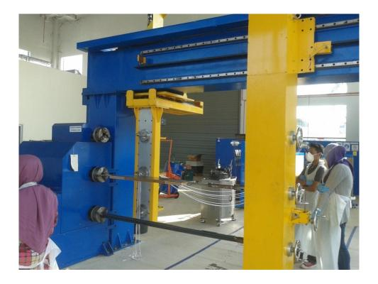
Figure 10: Customized filament winding machine in SIRIM Permatang Pauh
