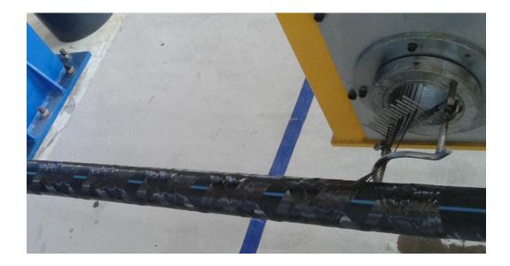
Figure 11: Helical winding process
