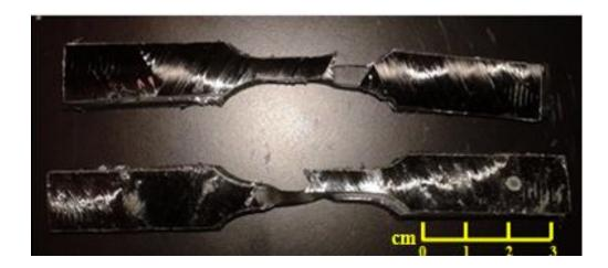
Figure 27: Dog-bone tensile sample
