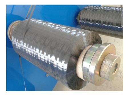
Figure 3: Sample 12K carbon fiber tow
