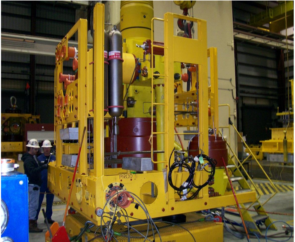
Figure 1 : Enhanced Vertical Deepwater Tree
