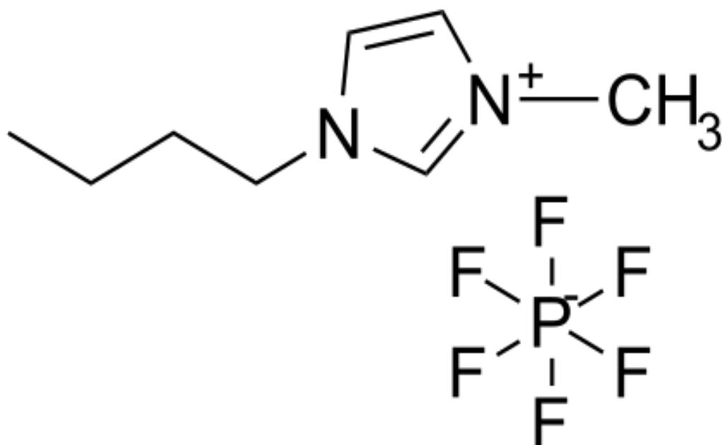
FIGURE 2.3.5. 1-butyl-3-methylimidazolium Hexafluorophosphate
