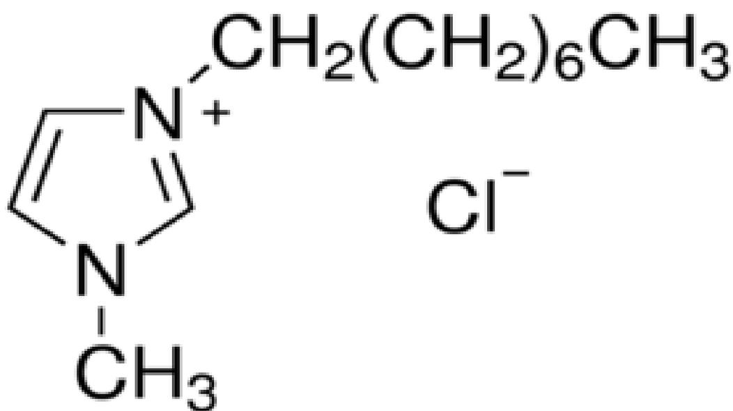
FIGURE 2.3.3. 1-methyl-3-Octylimidazolium Chloride
