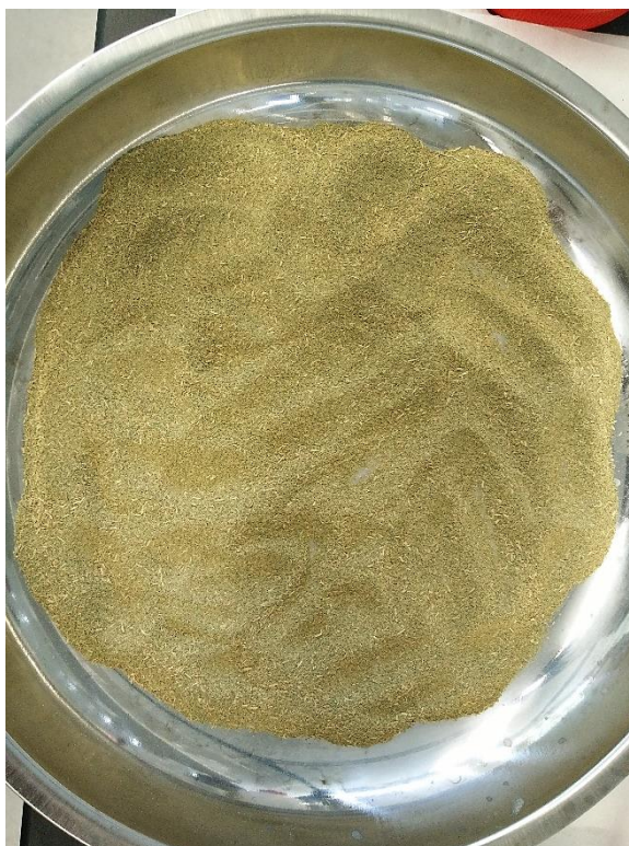
FIGURE 3.2 1-mm size tea tree powder after manual sieving
