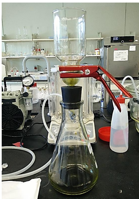
FIGURE 3.9 Vacuum filtration setup to separate waxes from essential oil
