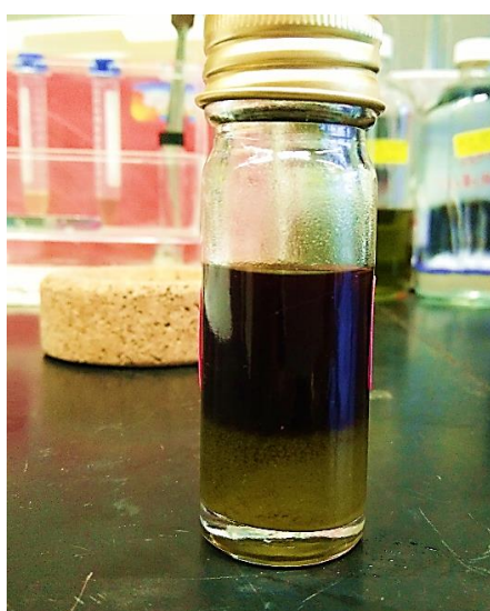
FIGURE 3.8 Precipitated waxes after mixture is cooled for 1 day
