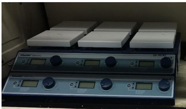
FIGURE 3.4 Digital Hotplate Magnetic Stirrer.
