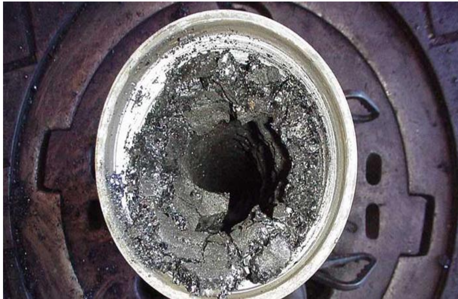
Figure 1.1: Deposition of asphaltene in tubing
