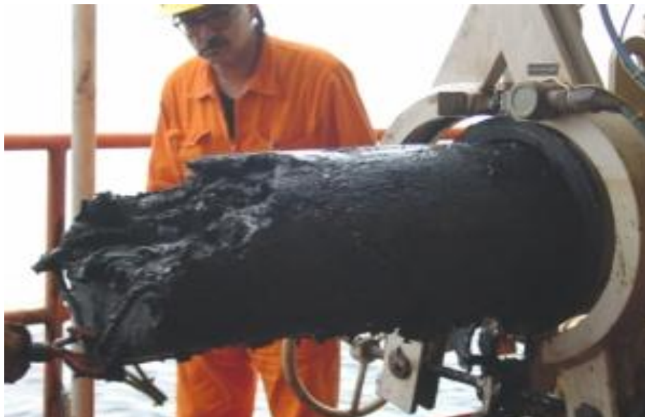
Figure 1.2: Asphaltene deposition cause pipe blockage
