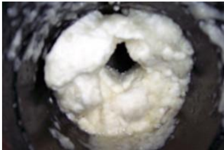
Figure 1.1: Solid crystalline compound of hydrates formed inside the pipeline (Alberta Analytical Ltd, 2013)
