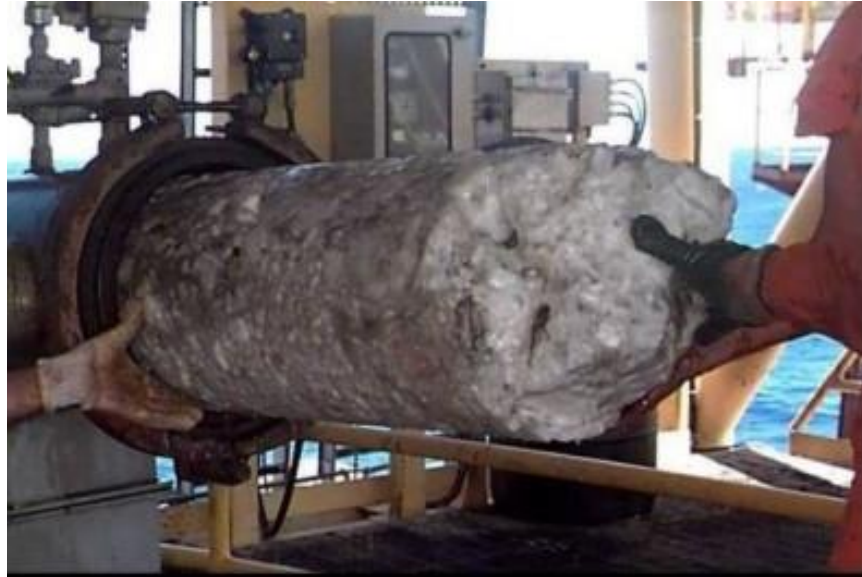
Figure 1.2: Removal of hydrates from pipeline during work-over operation (Heriot Watt Institute of Petroleum Engineering, 2015)
