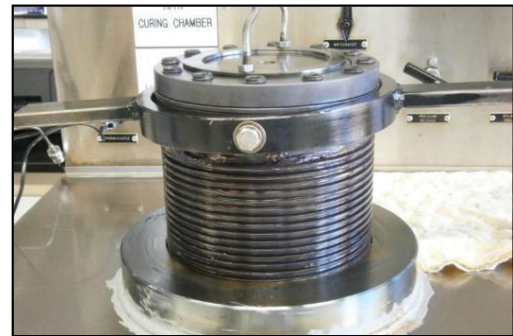
Figure 3-12: Moulds inserted into pressure vessel and cylinder plug threaded into it
