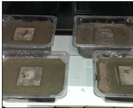
Figure 3-13: The cured cement sample is put into the cement holder
