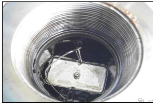
Figure 3-12: Moulds inserted into pressure vessel and cylinder plug threaded into it
