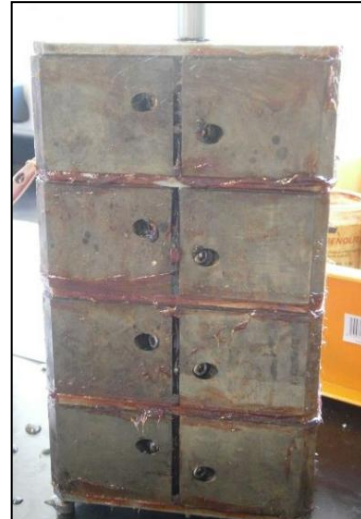
Figure 3-10: Cement slurry filled in mould Figure 3-11: Curing moulds stack up
