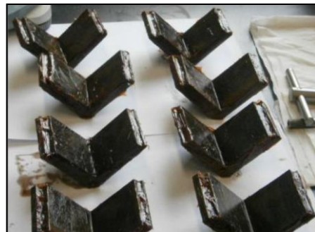
Figure 3-9: Greased curing moulds
