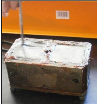
Figure 3-10: Cement slurry filled in mould Figure 3-11: Curing moulds stack up
