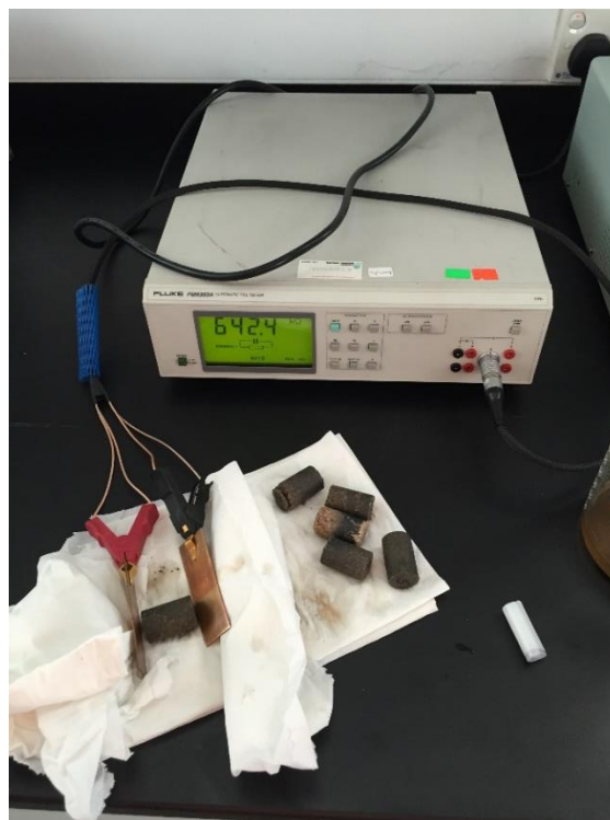
Figure 14 Measuring the Electrical Resistivity of Core Samples Using RCL Meter
