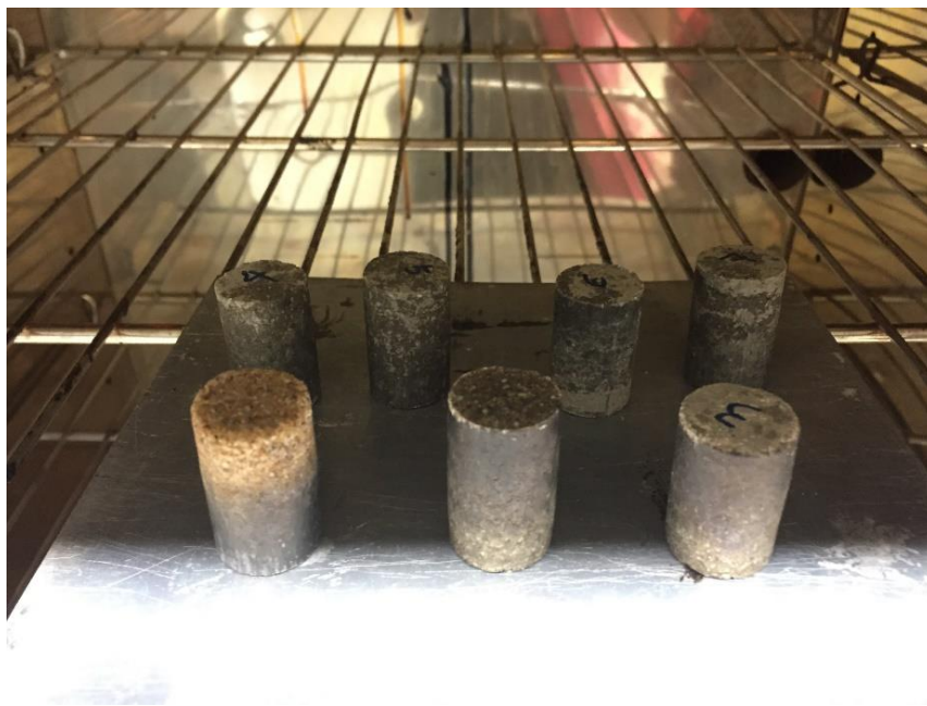
Figure 12 Heat Treatment of Core Sample in the Oven
