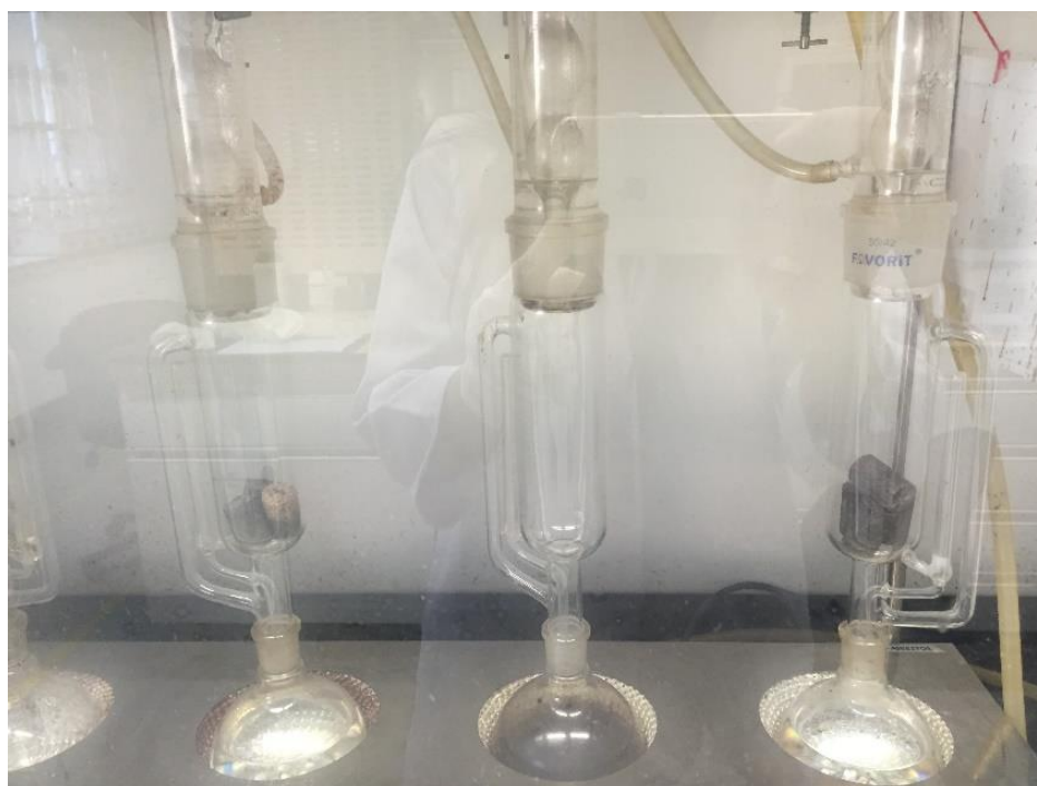
Figure 15 Cleaning of Core Samples from Salt Particles Using Soxhlet Extractor
