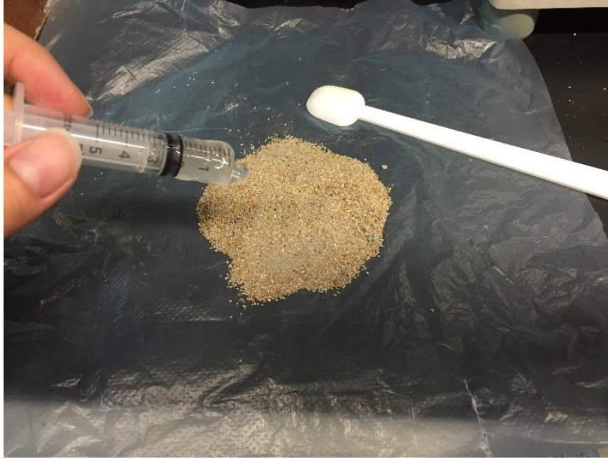
Figure 10 Adding Sodium Silicate Solution to the Mixture
