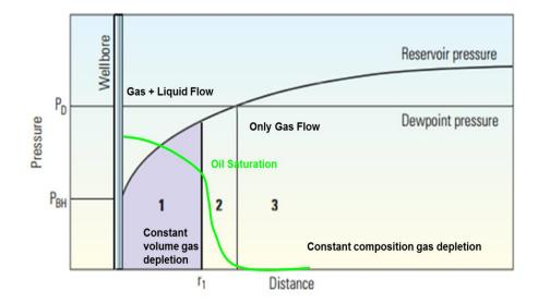
Figure 8: Pressure vs distance of Retrograde Gas Reservoir liquid build up analysis
