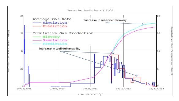
Figure 19: IPM MBAL results on average gas rate and cumulative gas production
