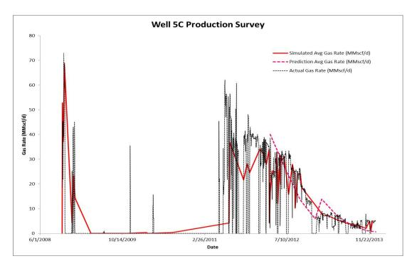
Figure 14: History matched, simulated, and prediction of gas production from IPM MBAL
