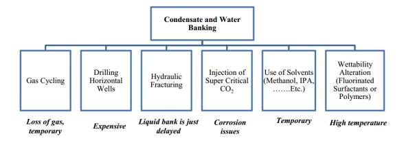
Figure 9: Summary of applicable technique in mitigating condensate banking
