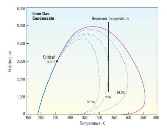
Figure 5: Phase diagram of a Lean Gas Condensate Reservoir (Fan et al., 1998)
