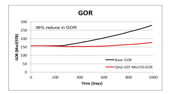
Figure 22: Gas Oil Ratio (GOR) changes upon propane injection
