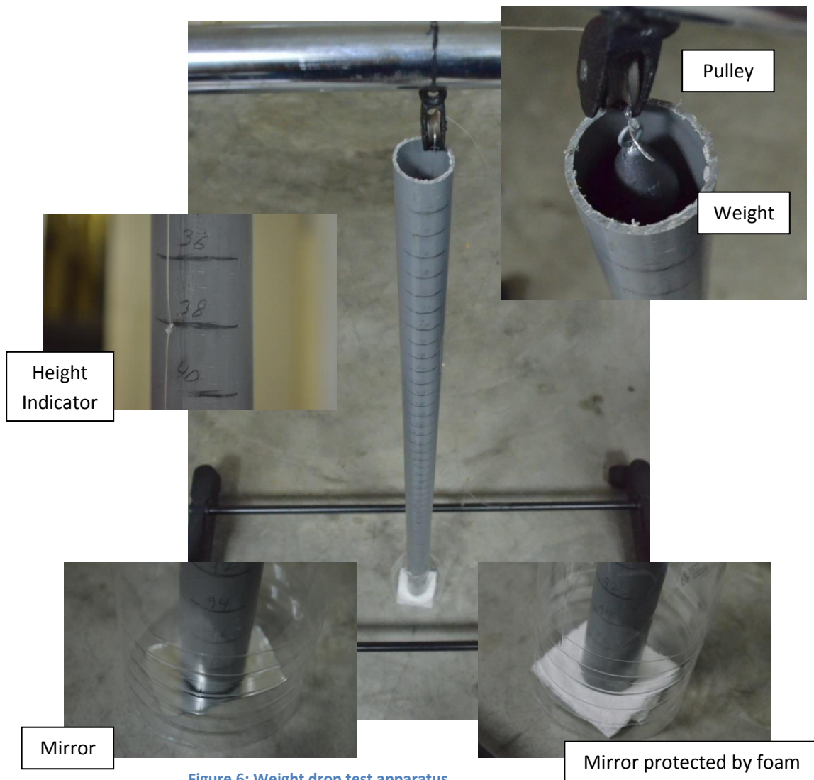
Figure 6: Weight drop test apparatus
