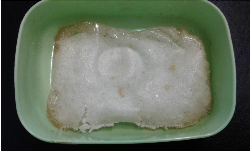
Figure 11: Foam started to degrade
