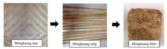
Figure 3.2: Sequence of mengkuang fibre preparation.
