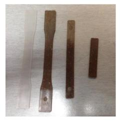
Figure 3.7 : Specimens produced by injection moulding.
