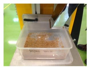
Figure 3.5: Pellets of PP/mengkuang fibre composite.
