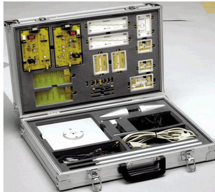
Figure 3.3 Microwave Communication Trainer kit
