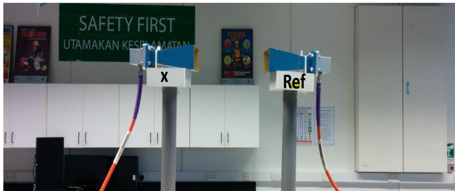
Figure A2: Setup for normalization to a reference antenna.
