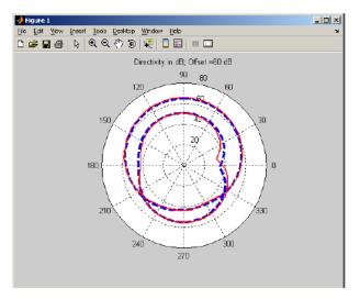
Figure 6: Result of directivity simulated by MAT (solid curve) and directivity predicted by ANSOFT HFSS (dashed curve)
