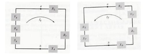
Figure 4: Thevenin equivalent of antenna in transmitting and receiving mode
