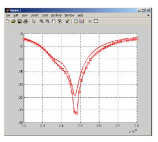
Figure 5: Result of antenna return loss simulated by MAT (squared curve) and return loss predicted by ANSOFT HFSS (solid curve)
