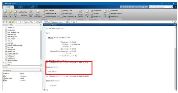
Figure 14: Directivity of antenna calculated with the azimuth and elevation as well as the frequency prompted from user
