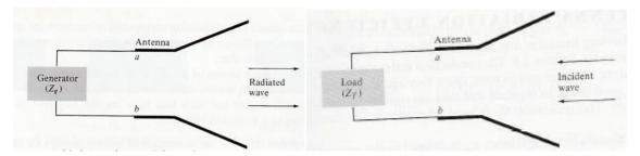
Figure 3: Antenna system in transmitting and receiving mode
