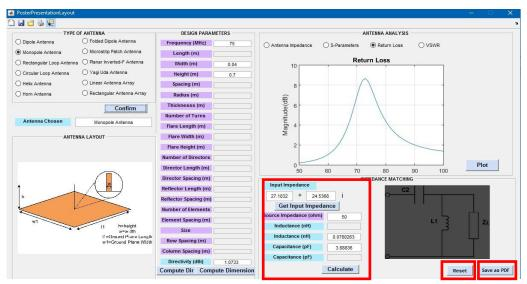
Figure 28: Impedance matching network is designed
