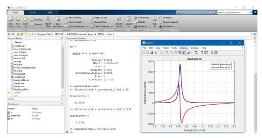
Figure 19: Input impedance of antenna calculated with the frequency range prompted from user
