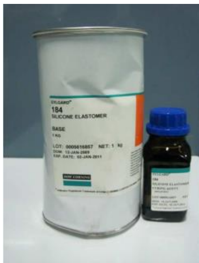
Figure 10: Dow Corning's Sylgard 184 elastomer kit, base and curing agent for the preparation of PDMS.
