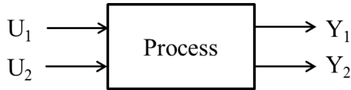
Figure 1: 2 \times 2 system block diagram.
