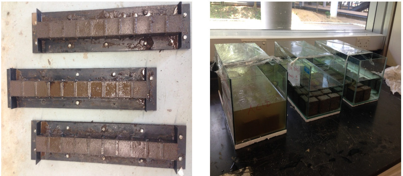
Figure 6: Moulding and Curing in Acid, Salt, and Normal water
