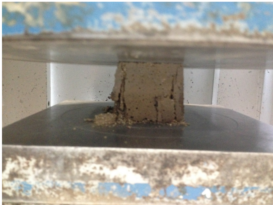
Appendix 4: Geopolymer mortar during compressive test
