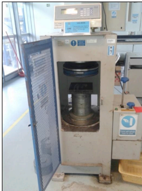
Figure 7: Compressive Strength Testing Machine
