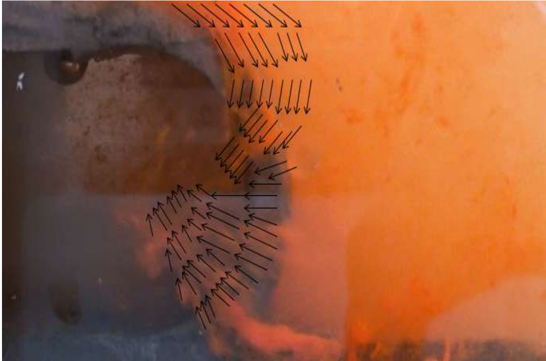
Figure 20 : Formation of Eddy on the Circle Breakwater at 13s
