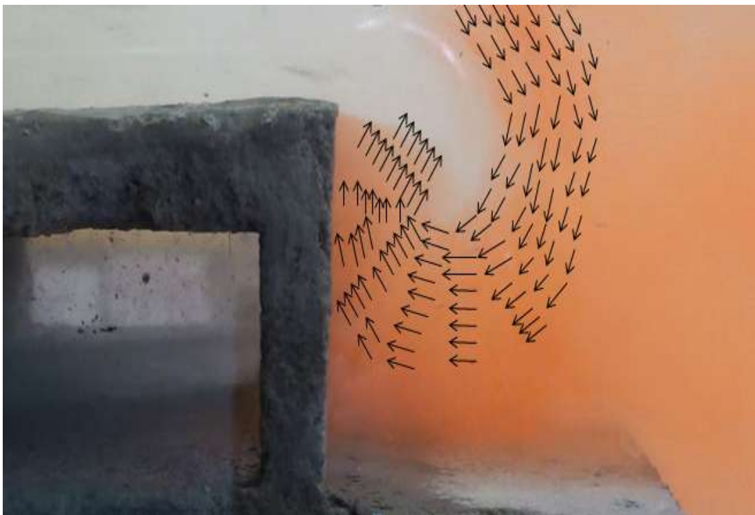
Figure 19 : Formation of Eddie on the Rectangular Breakwater at 13s
