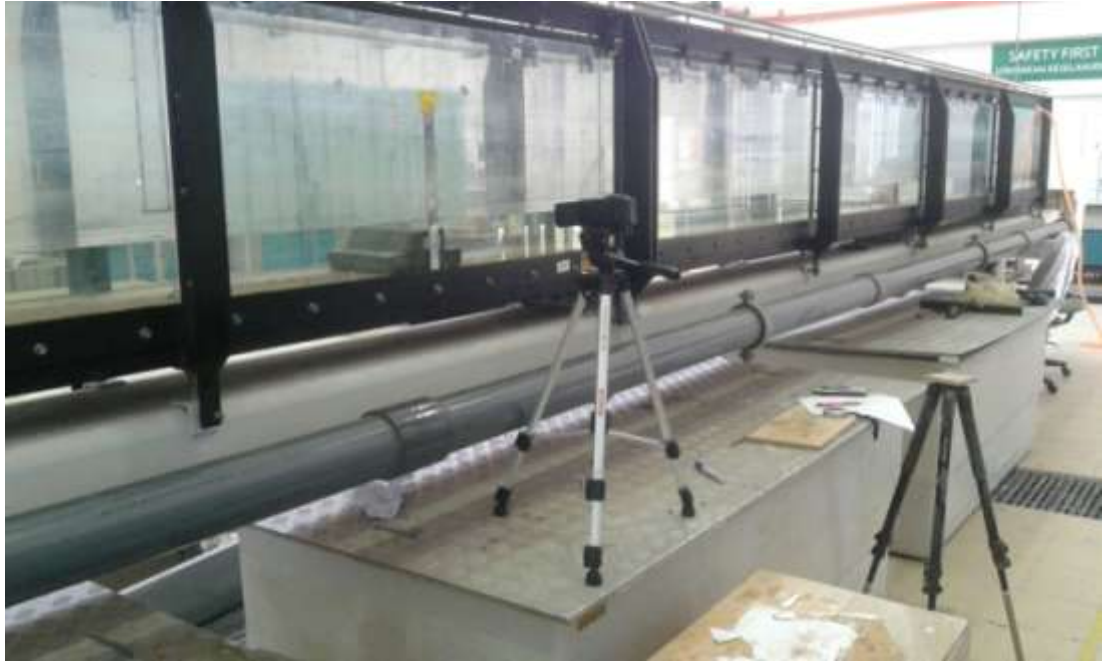
Figure 12 : The side view of breakwater in the HM 160 flume
