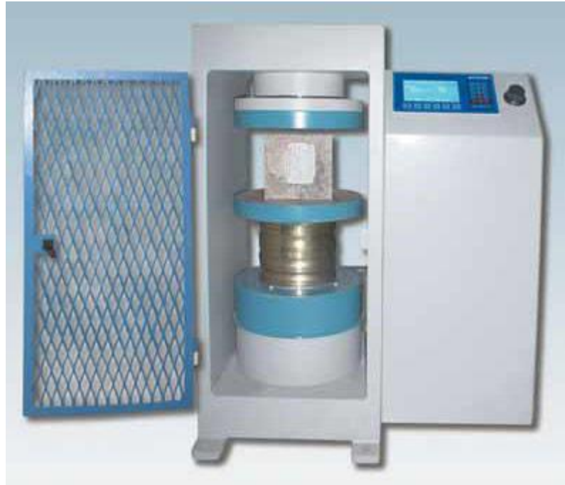
Figure 8: Compressive Strength Test Machine
