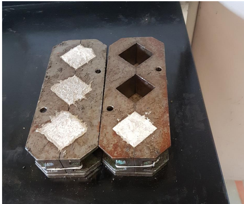
Figure 7: Mortar Cubes molds
