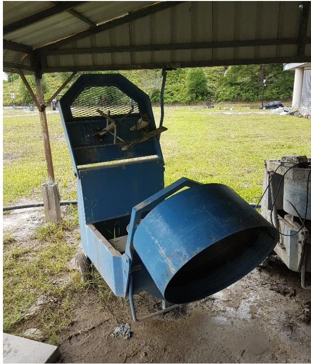
Figure 6: UTP concrete mixer
