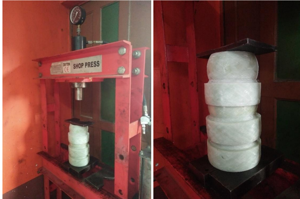
FIGURE 3.12: BALL SOCKET JOINTS BEING PRESSED
