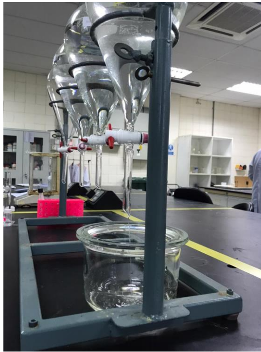
FIGURE 3.6 Solution separating process
