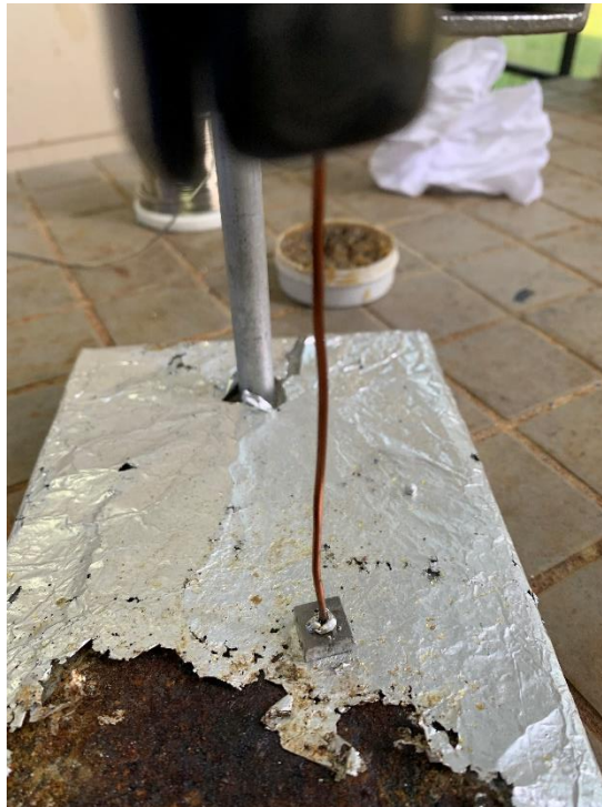
FIGURE 8. Copper wire connected to the sample by soldering
