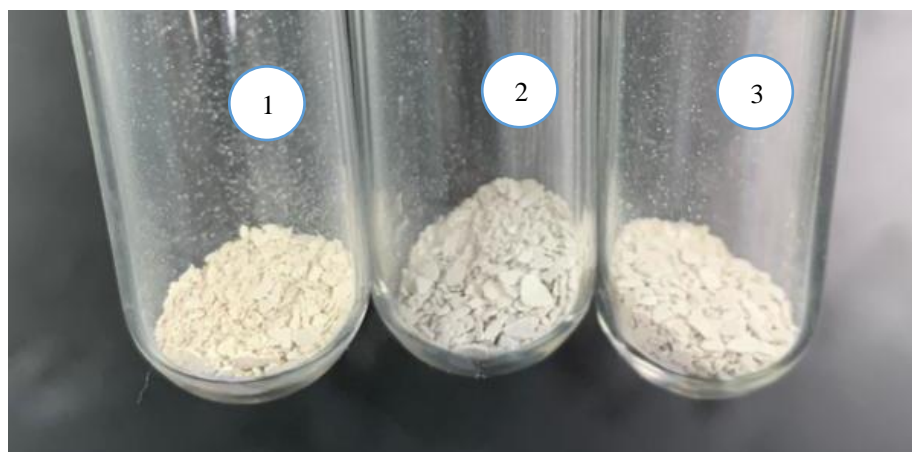
FIGURE 14. (1) 1g/l TO HNT (2) 1.5g/l TO HNT (3) 2 g/l TO HNT which Final product of thyme oil loaded HNT with vary concentration
