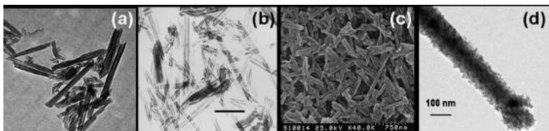
FIGURE 3. (a)(b)(c)(d) The FESEM image of layer-by-layer nanocoating HNT [1]
