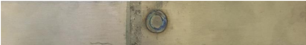
Figure 4.1 Top view of weld nugget for Ti-6Al-4V sample
