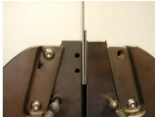
Figure 4.3 Spacer used to align the specimen with the machine during the tensile test
