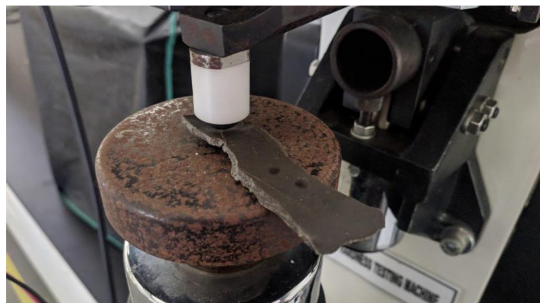
Figure 4. 3: Specimen failure during Rockwell Hardness Test
