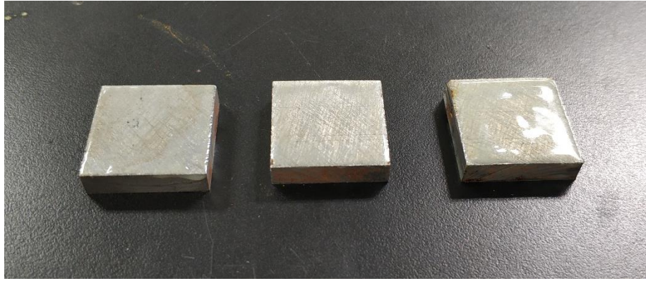
Figure 3.4: Metal plate applied with epoxy
