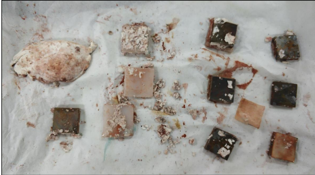
Figure 4.5: The samples after putting into autoclave machine
