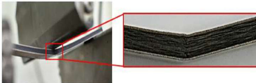
Figure 2.8: Specimen undergoing 3-point bending test [10]
