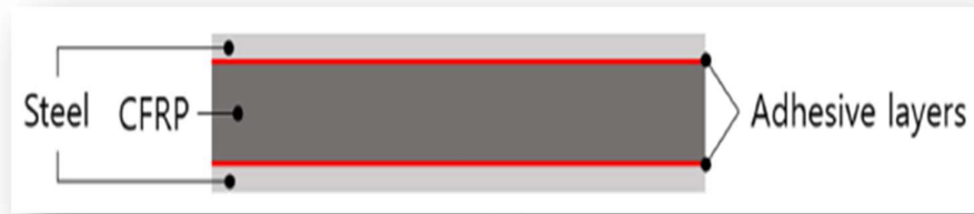
Figure 2.6: Carbon Fibre Reinforced Polymer (CFRP) core laminate material [10].
