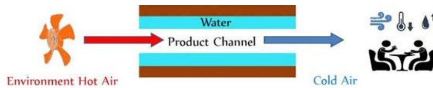
Figure 2.3: Direct Evaporative Cooling System
