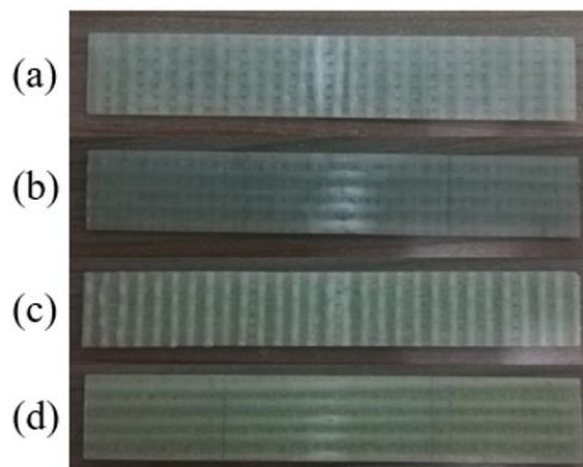
Figure 4.6: Macro-scale damage on rear surfaces of on-axis samples including thermosetting 0 degree sample (a), thermosetting 90 degree sample (b), thermoplastic 0 degree sample (c), and thermoplastic 90 degree sample (d)
