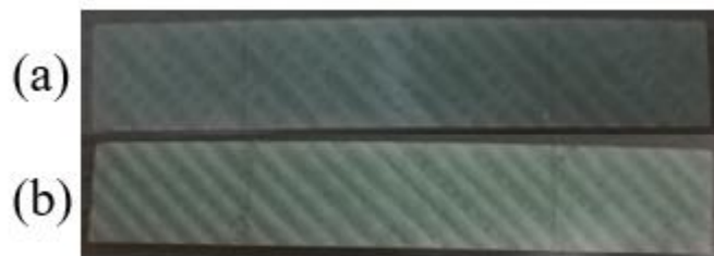
Figure 4.7: Macro-scale damage on rear surfaces of off-axis samples including thermosetting 45 degree sample (a), and thermoplastic 45 degree sample (b)
