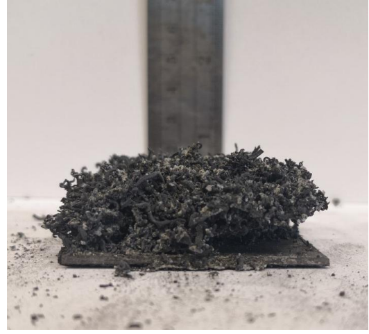
Figure 22: S004 after furnace test
