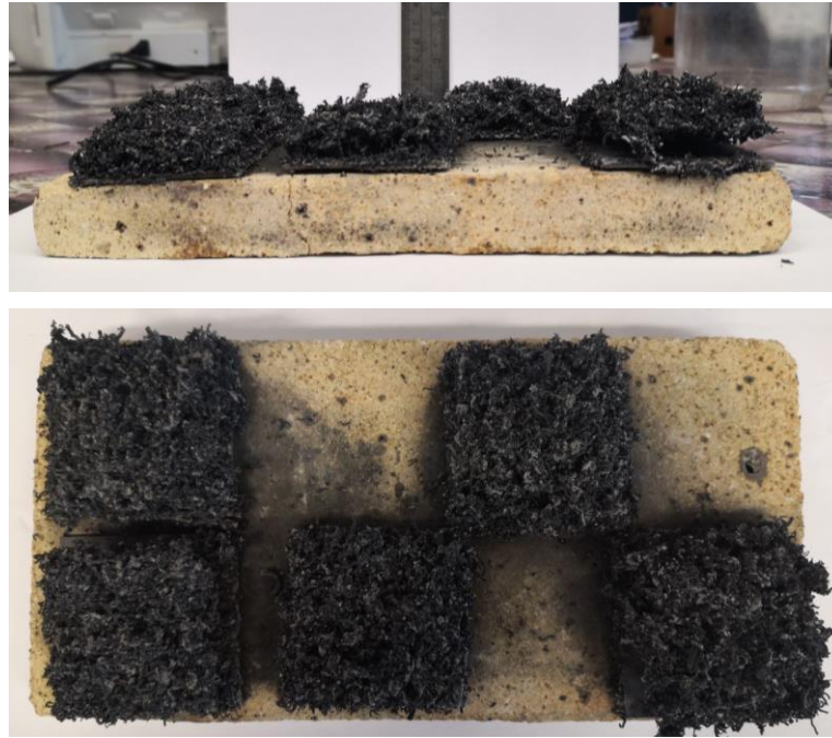
Figure 30: Second formulation samples after furnace test
