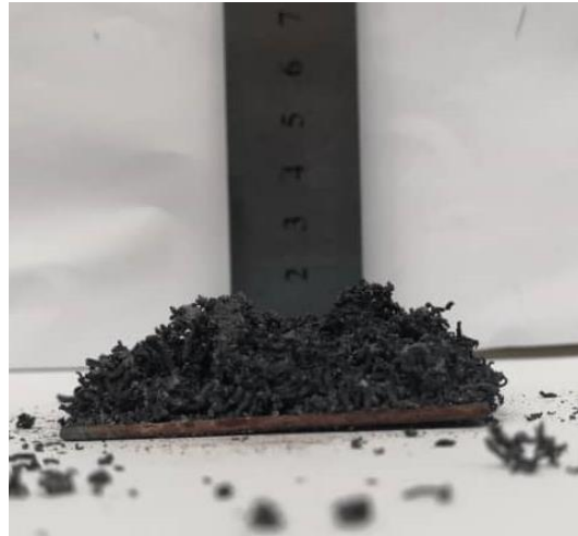
Figure 36: CF after furnace test
